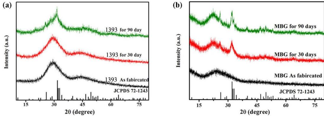
Fig. S1 XRD patterns for 1393 (a) and MBG (b) glass powder as immersed in SBF for 0 and 90 days. A reference hydroxyapatite (JCPDS 72-1243) is shown for comparison.
